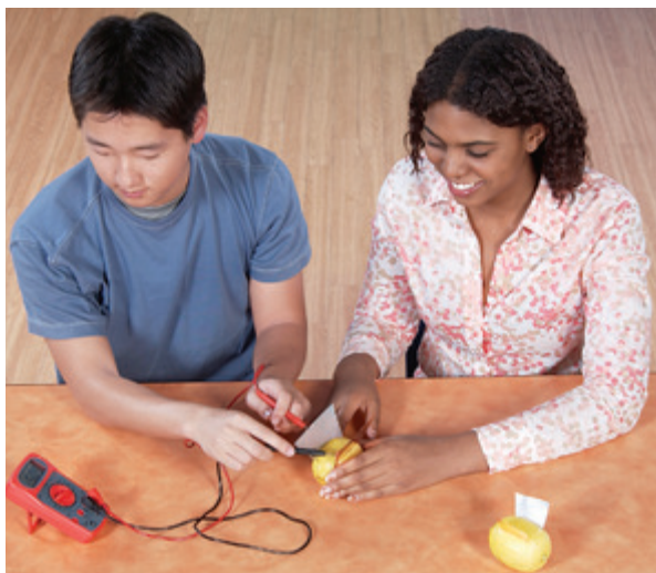
Figure 13 Batteries maintain electric current by converting chemical energy into electrical energy.
